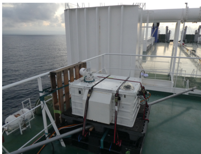
Figure 1. Box housing the EM27/SUN FTS, the DOAS spectrometer, and the sun tracker assembly. The box is positioned on the upper deck of the vehicle-carrier Nichiyu Maru (Ocean Link, Ltd.).
