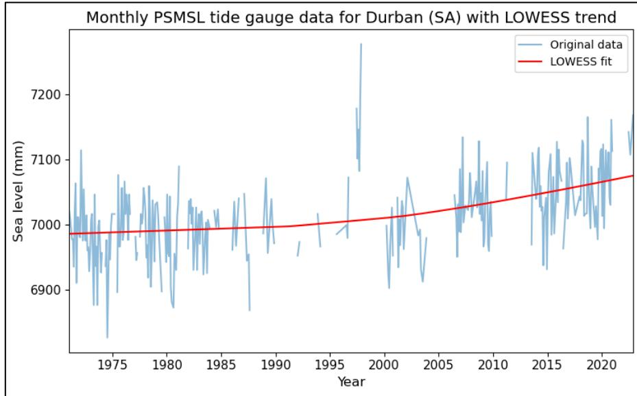
For our comparison, we assume equal SLR of the tide gauge data as at the start of the 30-year timeseries from Treu et al. (2024). Comparing the SLR at the time of event, we find the tide gauge data to result in a SLR of 119 mm compared to our SLR estimate of 96 mm. The tide gauge SLR value of 119 mm falls within the additionally included plausible range for SLR (150 mm).
