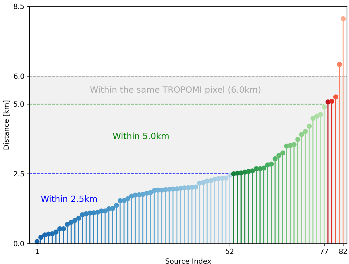
285 Figure 7. Distance between the actual and our detected locations of large Indian SO 2 point sources. The grid resolution of the emissions is 0.025° × 0.025° (approximately 2.5 km × 2.5 km per grid cell). Blue dots below 2.5 km: Detected and actual locations fall within the same grid cell. Green dots between 2.5 km and 5.0 km: Detected locations are in grid cells directly adjacent to the actual locations. Red dots above 5.0 km: Detected locations are in grid cells that are one grid cell further away from the actual
