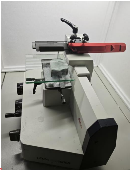
Figure A1. The Leica SM2000R microtome with a modified glass platform used in this study.
