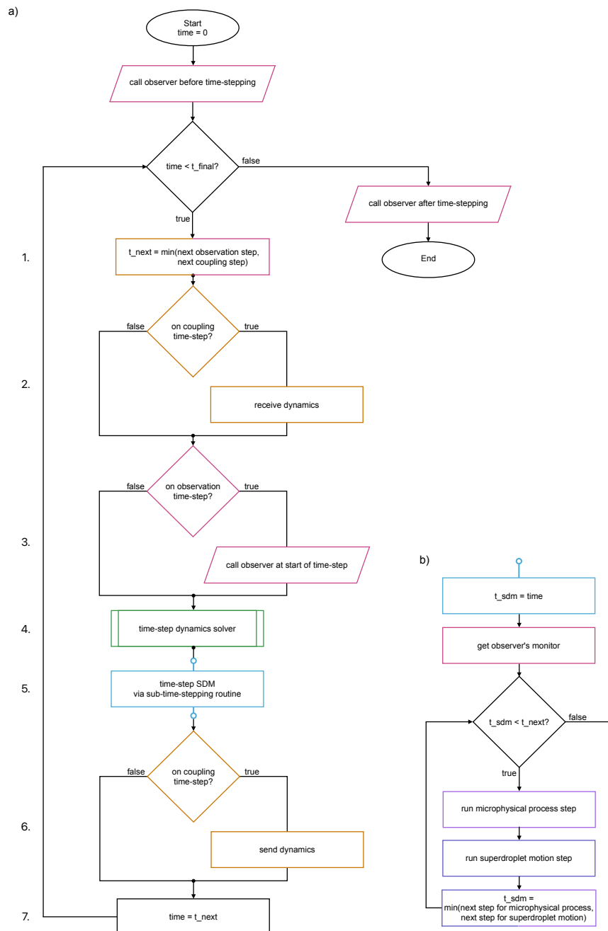
Figure 5. a) The flow diagram for CLEO's time-stepping routine. Each step is coloured by which of CLEO's structures it involves. The steps involved in the SDM sub-time-stepping routine are shown in b) and are an extension of the logic presented in Figure 4a to include output and superdroplet motion as well as microphysics.
