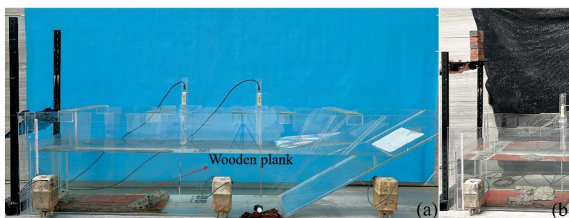
210 211 Fig. 3: Photographs of the setup, (a) Experimental flume, (b) platform for inducing 212 rotational cliff collapse.
