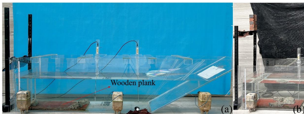
Fig. 3: Photographs of the setup, (a) Experimental flume, (b) platform for inducing rotational cliff collapse.
