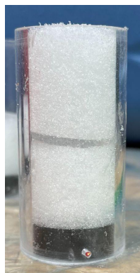
Figure 1. Ice lens sample. Snow was sieved into a 55 mm x 25 mm diameter container, and a 2 mm ice lens was situated midway with an approximately horizontal orientation.
