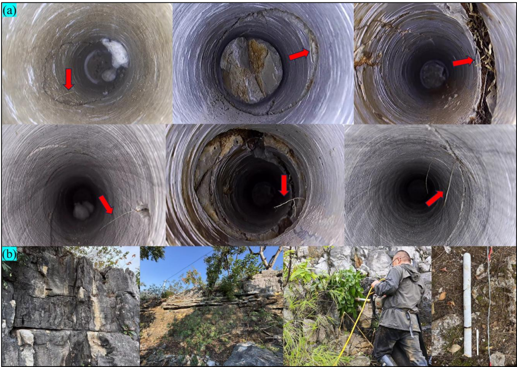
Fig. A4. Distribution of roots in rock fissure holes in exposed epikarst zones. We selected a number of epilithic karst zones with a thickness of more than 3 m to obtain rock fissure water by drilling diagonally downward from the base of the rock fissure (Fig. b). However, during the sampling period, we also detected the presence of a large number of roots within the holes (Fig. a).
