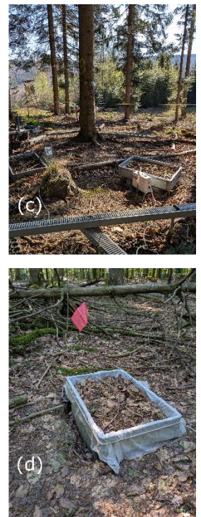
Figure 2: Design of FluxIT sampler with four equal drainage compartments (top view), each equipped with single tipping bucket units for measurement (cross section). Photographs (c, d) show samplers installed at two locations in the field, at a moment of configuration II for measurements of integrated throughfall with litter in the samplers
