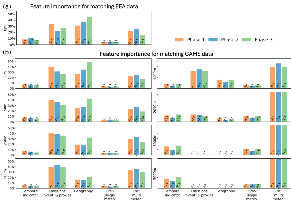
Figure 5. Relative importance of each input feature group for DACNO 2 model predictions, evaluated using the integrated gradients (IG) method. (a) Feature group contributions to RMSE between DACNO 2 surface NO 2 estimates and EEA ground-based measurements for 2023. (b) Feature group contributions to RMSE between DACNO 2 and CAMS NO 2 estimates at different vertical levels for 2023. The five feature groups are: temporal indicators, emission inventories and proxies, geography, ERA5 single-level meteorology, and ERA5 multi-level meteorology. Results are shown for each model training phase (Phase-1, Phase-2, and Phase-3), illustrating how the relative influence of input feature groups varies with training constraints and altitude. See Figure S3 for the contributions of individual features within each group.
