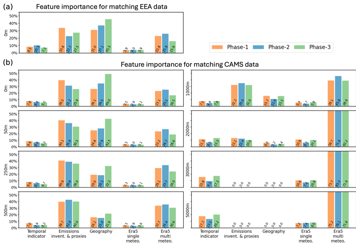
525 Figure 5. Relative importance of each input feature group for DACNO 2 model predictions, evaluated using the integrated gradients (IG) method. (a) Feature group contributions to RMSE between DACNO 2 surface NO 2 estimates and EEA ground-based measurements for 2023. (b) Feature group contributions to RMSE between DACNO 2 and CAMS NO 2 estimates at different vertical layers for 2023. The five feature groups are: temporal indicators, emission inventories and proxies, geography, ERA5 single-level meteorology, and ERA5 multi-level meteorology. Results are shown for each model training phase (Phase-1, Phase-2, and Phase-3), illustrating how the relative influence of input feature groups varies with training constraints and altitude. See Figure S9 for the contributions of individual features within each group. 530
