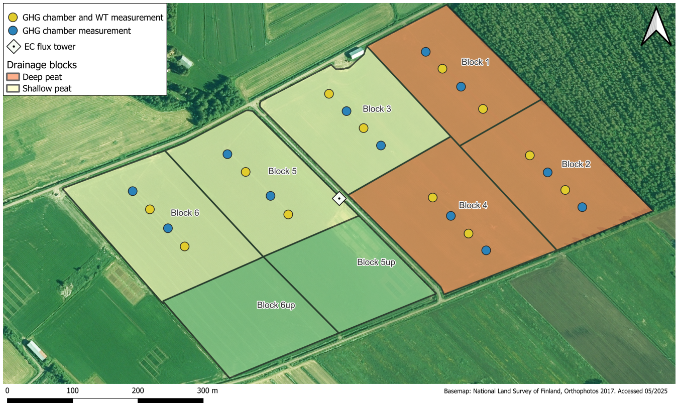
Figure 1. Study site with the different blocks highlighted by peat depth. Chamber measurements were done on blocks 1–6. EC measurements presented in this study include blocks 5, 6, 5up and 6up.
