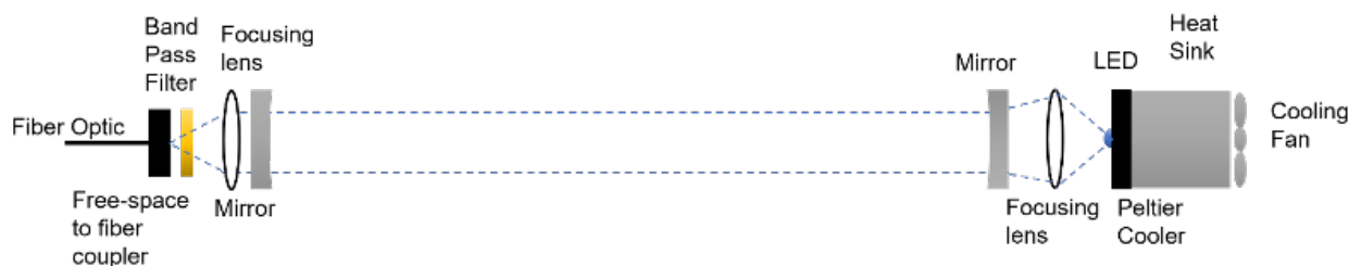
Figure 2. The BBCEAS cavity is comprised of a broadband light source coupled into an optical cavity consisting of two highly reflective mirrors, increasing the pathlength of the light. The transmitted light is collected and directed into a spectrometer via an optical fibre, where it is dispersed and recorded using a CCD detector.
