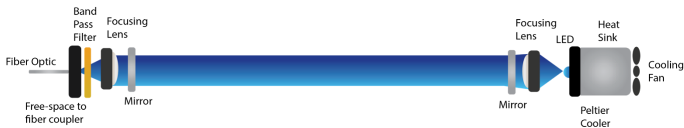
Figure 2. The BBCEAS cavity is comprised of a broadband light source coupled into an optical cavity consisting of two highly reflective mirrors, increasing the pathlength of the light. The transmitted light is collected and directed into a spectrometer via an optical fibre, where it is dispersed and recorded using a CCD detector.
