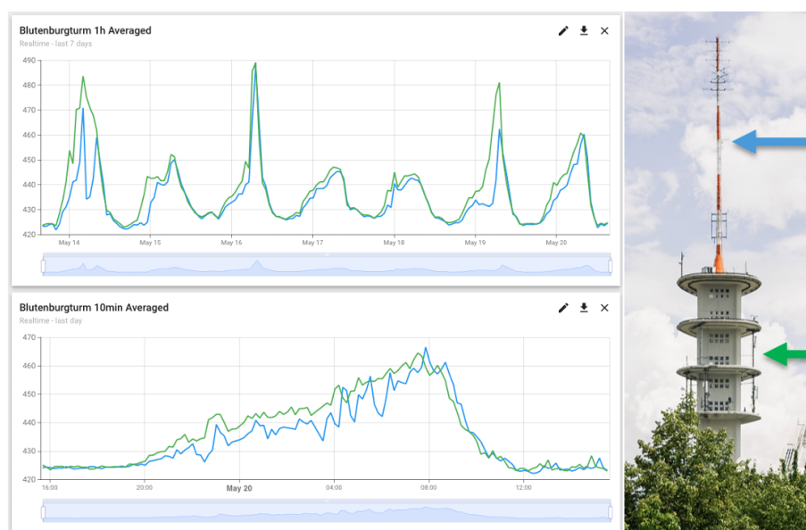
Figure 11. Time series of CO 2 concentrations at two heights at the BLUT tower for a week in May 2025. Measurements from the ACROPOLIS network are shown for inlets at 48 m (green) and 85 m (blue) above ground level. Data are taken from the live ThingsBoard dashboard and illustrate typical vertical gradients under varying atmospheric conditions. The image shows the measurement inlet positions at the Blutenburg Tower (photo by @ICOS_RI)
