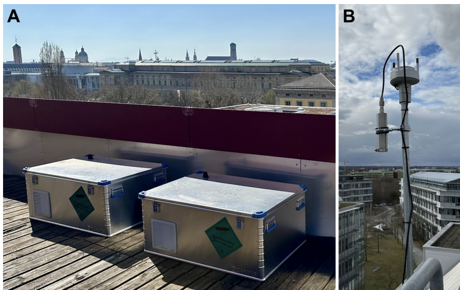
Figure 2. (A) Two ACROPOLIS outdoor enclosures deployed on the university rooftop site (TUMR). (B) Air inlet and co-located Vaisala WXT-532 wind sensor mounted on a pole at the GROR site.
