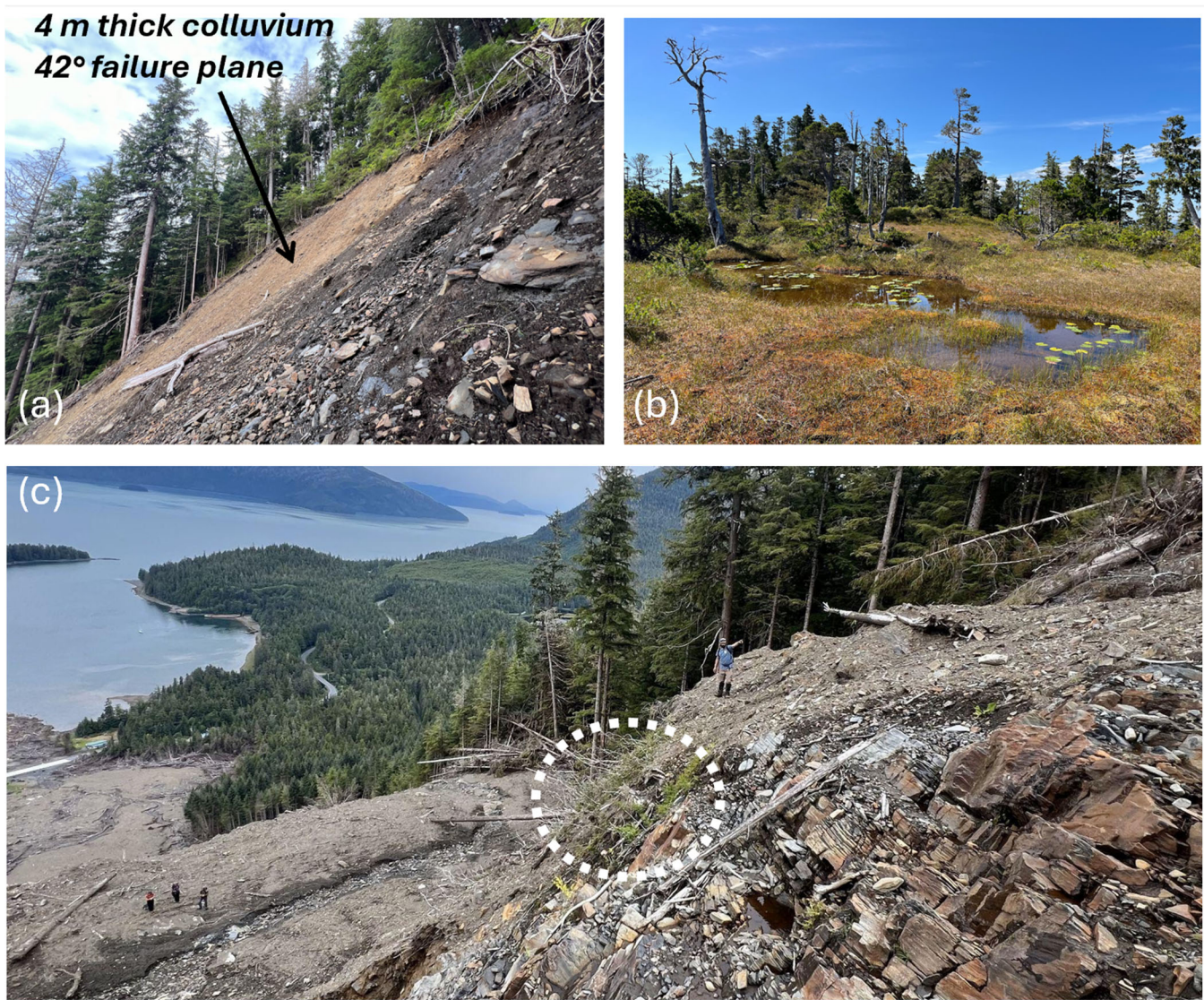
Figure 9. Photographs of key features identified in the field: (a) view to the north across the head scarp, exposing thick colluvial wedge in lateral margin, (b) ridgetop wetland or muskeg that drains to the head scarp, and (c) oblique view of mid-slope location (~1,000 m on transect; see Fig. 11) depicting high relief and resistant cliff-forming unit and patch of live blueberry bushes denoted by dashed white circle just below the top of the bedrock cliff. Note person for scale.
