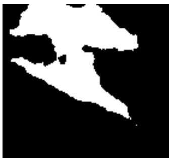
Figure 15. Binarized and inverted image of the score matrix used to mask the background tracer in the background analysis for the urban-scale application.
