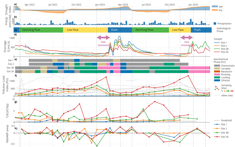
580 Figure 3: Water and metal transport regime in the Reiche Zeche mine. (a) Dryness index as an indicator of the general water 581 situation on the surface. (b) Weekly precipitation collected from Reiche Zeche, Freiberg weather station. (c) Hydrologically defined 582 flow phases. (d) Discharge at the four sites in the Reiche Zeche mine. Pink arrows represent time periods when hot moments occur. 583 (e) Geochemical hysteresis phases of pollution load index (PLI) at the four sites. (f) PLI dynamics. (g) CV_c/CV_q ratios (with a 584 threshold of 0.5), and (h) Hysteresis Area from the HARP method are shown across the mine system. Individual sites are connected 585 by black lines and colored lines are monitored flow sites for sites 1, 2, 3A, and 3B.
