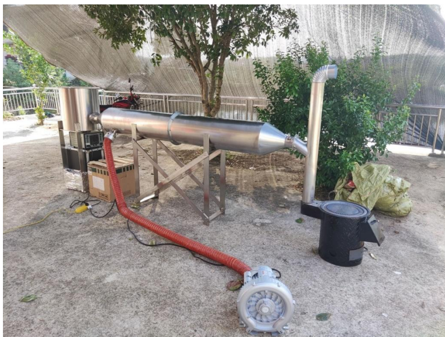
Figure S2. A photo of the apparatus used in our work to collect aerosol particles emitted by domestic coal and biofuel burning.
