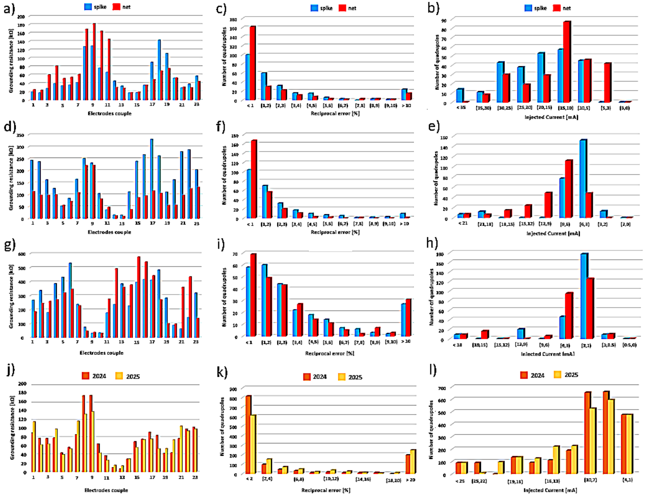
Figure 2. Histograms (a), (d), and (g) compare grounding resistances [kΩ] recorded at the Marocche di Drò, Sadole, and Flüela test sites, respectively, using traditional stainless-steel spike electrodes with sponges (blue) and the proposed stainless-steel net electrodes with sponge inserts (red). Panels (b), (e), and (h) show the corresponding injected electric currents [mA], while (c), (f), and (i) present the reciprocal error [%] of the quadrupoles for the same sites and electrode types. All electrodes were moistened with the same amount of saltwater and placed at comparable positions between surface boulders (see Fig. 1b–c). Panels (j), (k), and (l) illustrate the contact resistances (first 24 electrodes, as in panel a), injected currents, and reciprocal errors for datasets acquired at the Sadole site in June 2024 (orange) and June 2025 (yellow) along the permanent ERT monitoring line using the stainless-steel net electrodes.
