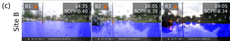
Figure 3: (a) SOFI time series for 14 May moderate severity case study event. Representative flooded images from (b) Site A and (c) Site B. Segmented flood masks are shown in blue.
