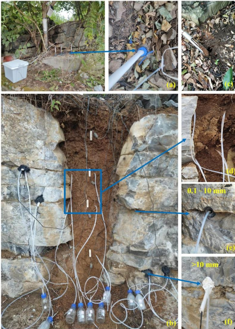
Figure A1. Field photographs illustrating soil and rock water sampling procedures. (a) Vertical boreholes drilled at sites C, D, and E with water sampling devices installed at predefined depths. (b) Horizontal boreholes drilled into exposed bedrock outcrops at sites A and B with sampling devices installed within the soil-rock profile. (c) Collection of soil samples for laboratory extraction of bulk soil water. (d) Collection of mobile soil water using suction lysimeters installed in soil layers. (e) Collection of rock fracture water from narrow fractures (aperture approximately 0.1–10 mm) with little or no soil infill. (f) Collection of infilled rock fracture water from wider fractures (>10 mm aperture) largely filled with soil or fine sediments.
