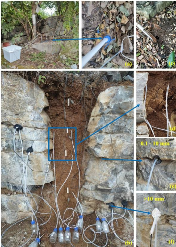
Figure A1. Field photographs illustrating soil and rock water sampling procedures. (a) Vertical boreholes drilled at sites C, D, and E with water sampling devices installed at predefined depths. (b) Horizontal boreholes drilled into exposed bedrock outcrops at sites A and B with sampling devices installed within the soil-rock profile. (c) Collection of soil samples for laboratory extraction of bulk soil water. (d) Collection of mobile soil water using suction lysimeters installed in soil layers. (e) Collection of rock fracture water
