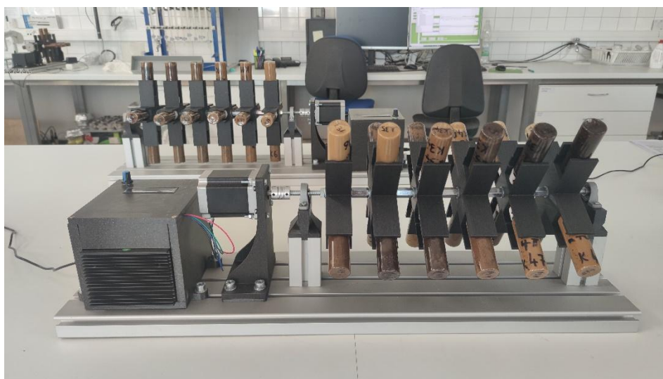
Figure A1: Custom-built laboratory apparatus designed to ensure homogeneous mixing of soil and added water through controlled mechanical motion of sealed sample vials prior to analysis.
