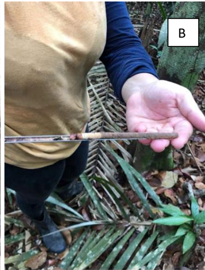
Supplementary Figure 5 Illustrative image of the Pressler drill embedded in a tree (A); sample obtained with the Pressler drill (B) to determine wood density
