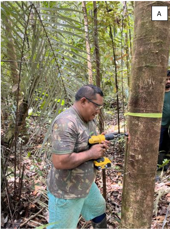
Supplementary Figure 4: The first image is a photo of the collection of woody material in the field with a 25 mm diameter drill attached to a drill press (A), in the second image we have a photo of the drill used (B)
