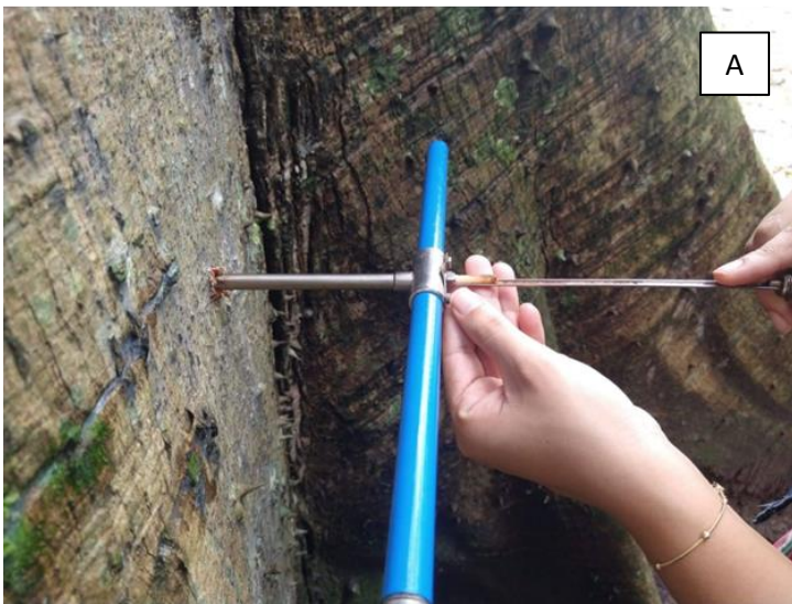
Supplementary Figure 5 Illustrative image of the Pressler drill embedded in a tree (A); sample obtained with the Pressler drill (B) to determine wood density
