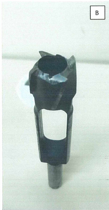
Supplementary Figure 4: The first image is a photo of the collection of woody material in the field with a 25 mm diameter drill attached to a drill press (A), in the second image we have a photo of the drill used (B)
