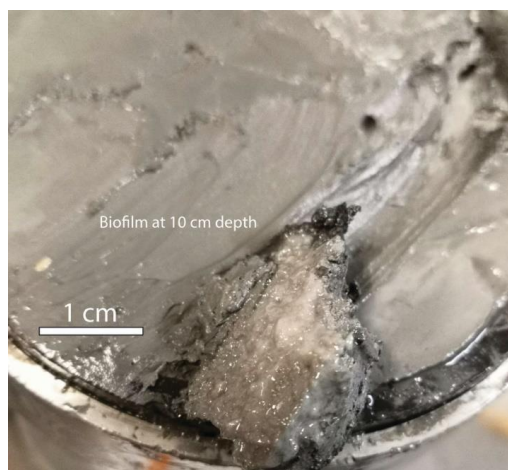
Figure 5. Photograph of a white biofilm encountered at 10 cm while slicing PusC-08. The sediment was sampled every cm in the interval 0-10 cm for microbiological analyses.
