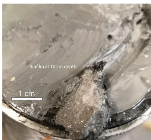
Figure 5. Photograph of a white biofilm encountered at 10 cm while slicing PusC-08. The sediment was sampled every cm in the interval 0-10 cm for microbiological analyses.
