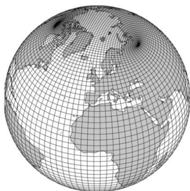
Figure 2 Tripolar (3600x2700) horizontal grid . Every 40 th gridpoint shown. Note that grid cells are approximately isotropic. credit: Mats Bentsen, GFDL.
