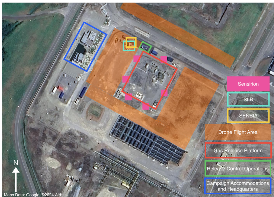
75 Figure 1. Map of the TADI test site. The gas release platform is indicated in red, the gas release control room in green, and the campaign headquarters in blue. Approximate location of the fixed sensors from Sensirion, SLB, and Sensia are indicated as well as common paths for drone flights.
