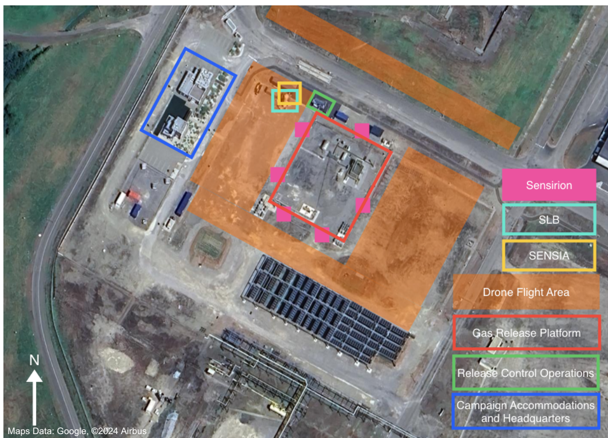
Figure 1. Map of the TADI test site. The gas release platform is indicated in red, the gas release control room in green, and the campaign headquarters in blue. Approximate location of the fixed sensors from Sensirion, SLB, and Sensia are indicated as well as common paths for drone flights.
