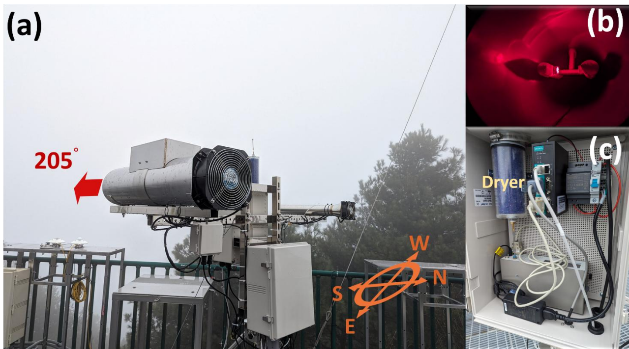
Figure 1: (a) The setup and Orientation diagram of Aerosol-Cloud Microphysics Monitoring System deployed at LABS during the 2024 observation period. (b) The appearance of CDP. (c) The appearance of 11-D.
