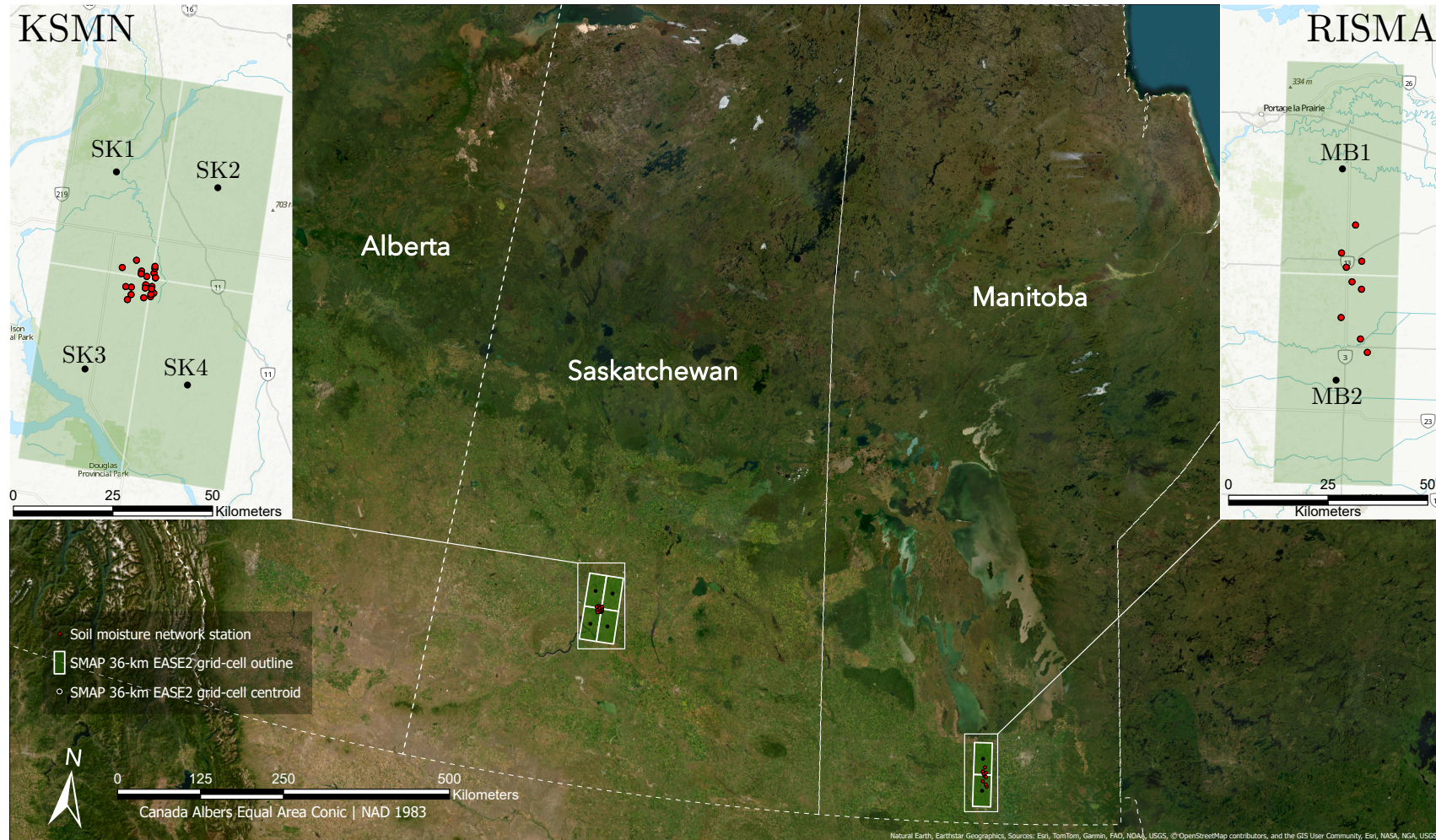
Figure 6: Figure R5. Study area map showing the Saskatchewan (KSMN) and Manitoba (RISMA) sites. Green rectangles: SMAP 36 km EASE-Grid pixel boundaries for the analysed pixels (SK1–SK4; MB1–MB2). Red dots: in situ soil moisture network stations. Insets show expanded views of each network. Projection: Canada Albers Equal Area Conic (NAD 1983).
