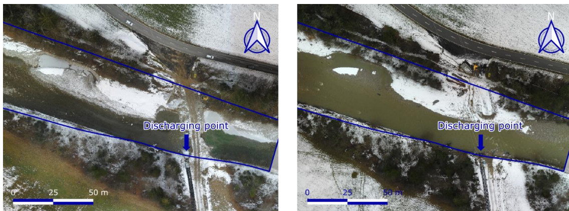
Figure A2. Snapshot of the pipes releasing pumped groundwater in the Emme River at two different flow scenarios (background image captured on site by the drone).
