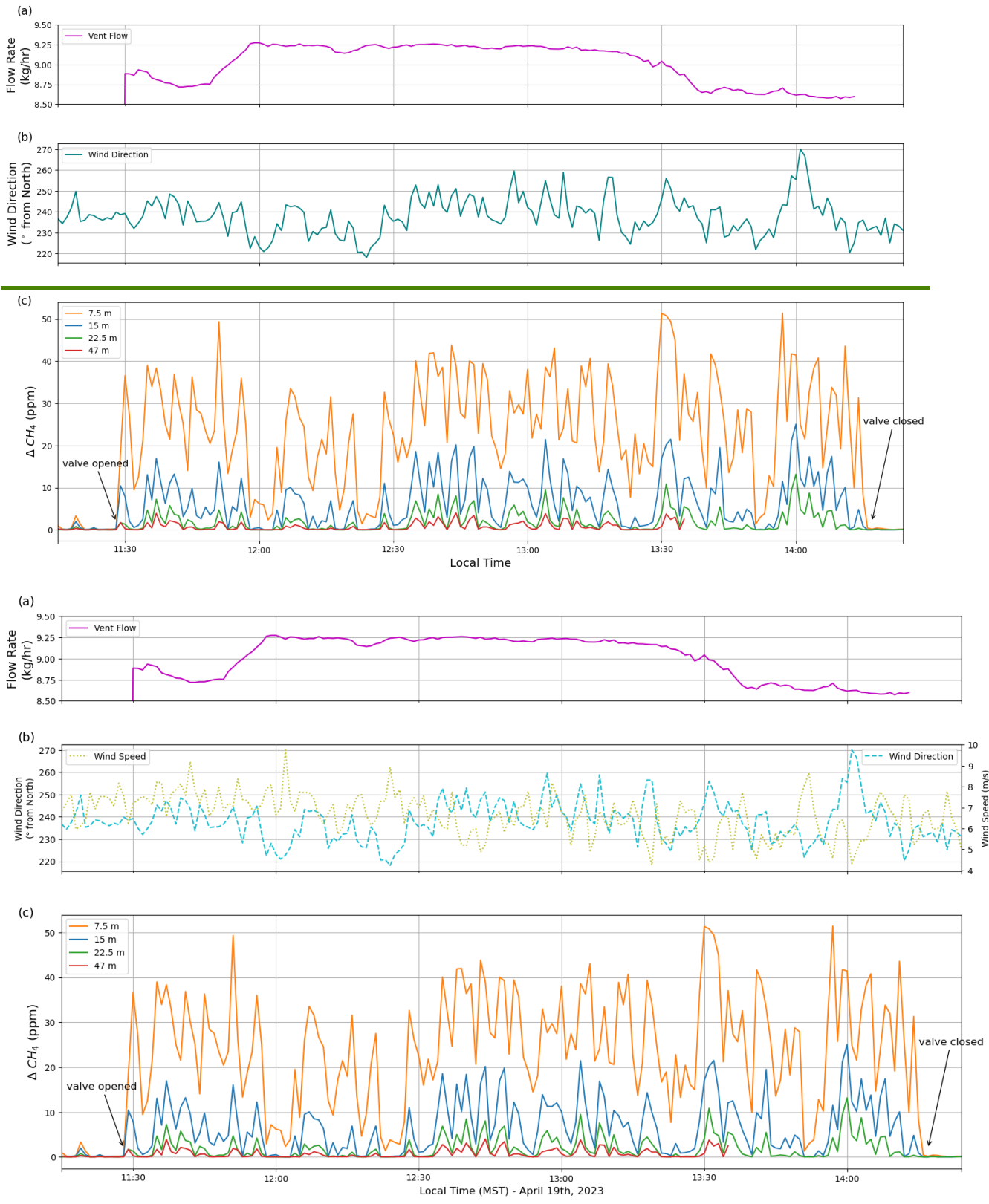
Figure 4: (a) Results of the methane release rate from Foster 1S well during venting as measured by Well Done using a Ventbuster flow meter. (b) Time series of the wind direction as measured by the TriSonica anemometer at 7.5 m downwind of the well site. (c) Results of the methane enhancement at 7.5 m, 15 m, 22.5 m, and 47 m.
