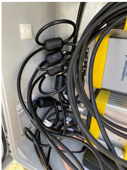
Figure 13. Installation of ferrites around the cables to suppress high frequency electronic noise.
