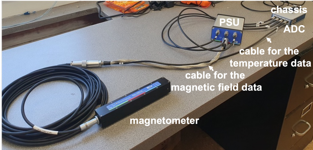
Figure 1. The elements comprising the instrumentation system of our geomagnetic variometer station, assembled in our lab. The magnetometer is a three-axes fluxgate Bartington Instruments magnetometer and is powered by a Bartington Instruments power supply unit (PSU). The data acquisition module (DAQ) is a NI-9239 from National Instruments, which contains an analog-to-digital converter. The output digital data are collected by a NI cDAQ-9171 (chassis), which is connected via USB to a mini PC by Intel (not shown here). See text for more details.
