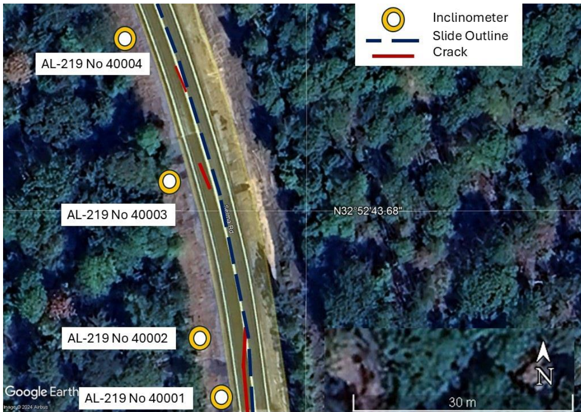
Figure 4. Location of four inclinometers at AL-219 site in Centerville and cracks caused by landslide, AL (Base map from ©Google Earth 2025).
