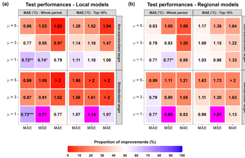
Figure 2: Median test performances (MAE, in °C) of the local models (a) and the regional models (b) according to the loss function used for training. These median values were computed from a set of 21 \times 4 = 84 points for the local models and 21 \times 7 = 147 points for the regional models. Note that the models we kept for test do not necessarily share the same lookback. Colours indicate the proportion of cases for which the use of the loss function yielded better results than the reference loss function (MSE with standardization, shown in magenta). Asterisks indicate that the custom loss function is significantly better than the reference loss function according to the binomial test: * for a significance threshold of 5%, ** for a threshold of 1%, and *** for a threshold of 0.1%.
