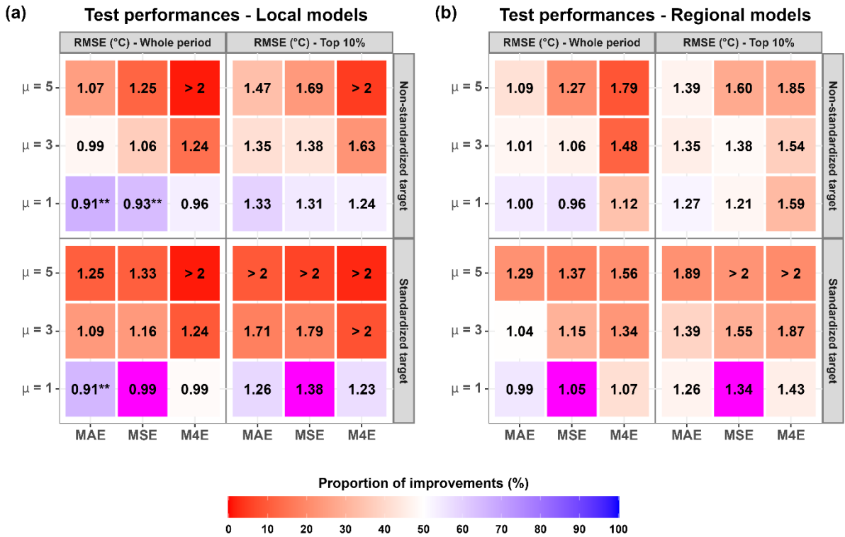
Figure R1: Median test performances (RMSE, in °C) of the local models (a) and the regional models (b) according to the loss function used for training. This figure is similar to Fig. 2 but with RMSE as a criterion to evaluate test performances. Colours indicate the proportion of cases for which the use of the loss function yielded better results than the reference loss function (MSE with standardization, shown in magenta). Asterisks indicate that the custom loss function is significantly better than the reference loss function according to the binomial test: * for a significance threshold of 5%, ** for a threshold of 1%, and *** for a threshold of 0.1%.
