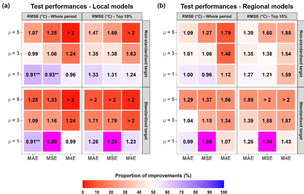
Figure R2: Median test performances in terms of RMSE (in °C) of the local models (a) and the regional models (b) according to the loss function used for training. Colours indicate the proportion of cases for which the use of the loss function yielded better results than the reference loss function (MSE with standardization, shown in magenta). Asterisks indicate that the custom loss function is significantly better than the reference loss function according to the binomial test: * for a significance threshold of 5%, ** for a threshold of 1%, and *** for a threshold of 0.1%.
