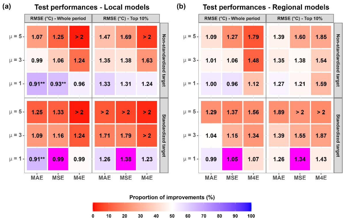
Figure R2: Median test performances in terms of RMSE (in °C) of the local models (a) and the regional models (b) according to the loss function used for training. Colours indicate the proportion of cases for which the use of the loss function yielded better results than the reference loss function (MSE with standardization, shown in magenta). Asterisks indicate that the custom loss function is significantly better than the reference loss function according to the
