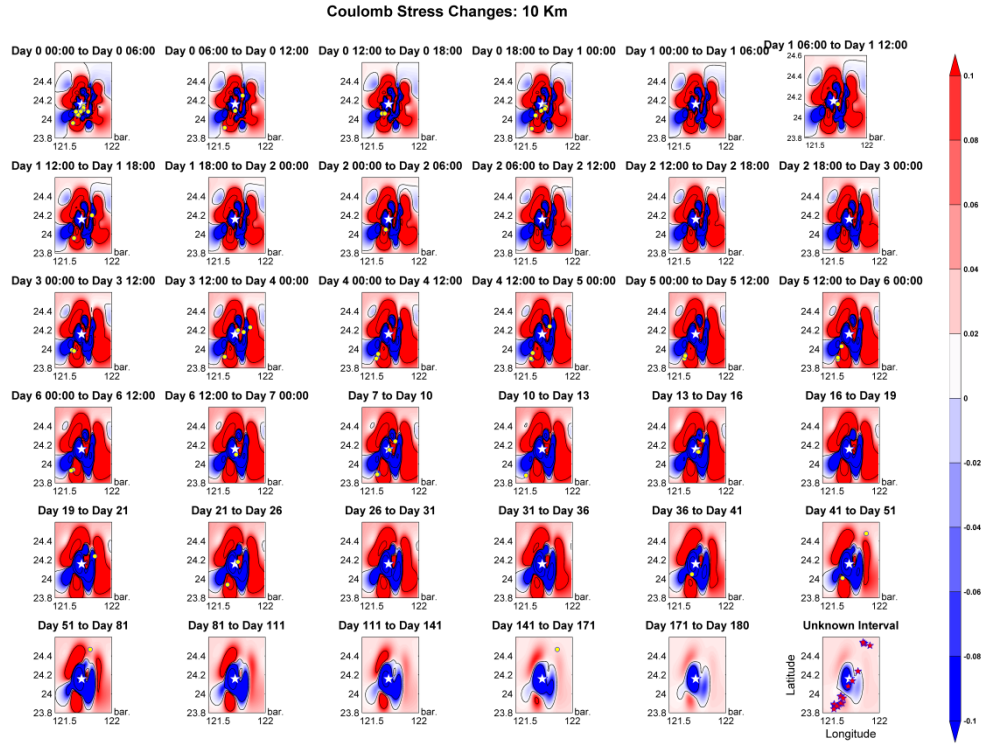
910 Figure A3: Temporal evolution of Coulomb stress changes at a depth of 10 km during the first 180 days following the 2018 Hualien earthquake (Mw 6.4). Each panel represents the Coulomb stress changes distribution over specific time intervals, with red regions indicating positive stress changes (stress loading) and blue regions indicating negative stress changes (stress unloading). The contours highlight the areas (>0.1bar) of significant stress concentration. The yellow circles indicate the epicenters of aftershocks occurring within 180 days of the mainshock, while the red stars in the final panel represent those occurring 2 to 3 years after the 915 mainshock.
