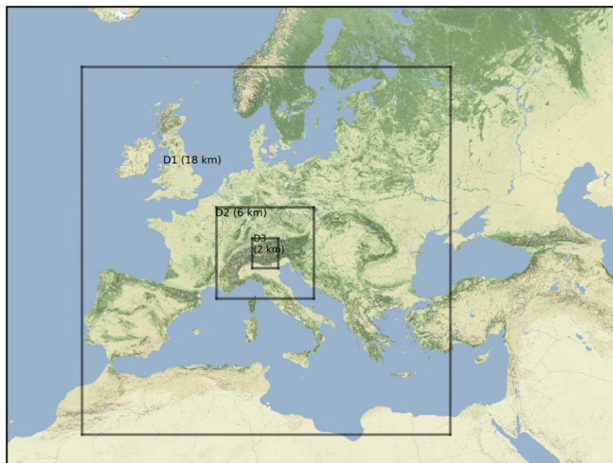
Figure 1: Dynamical downscaling with WRF is performed in three nested domains, with a grid spacing of 18 km (domain 1), 6 km (domain 2), and 2 km (domain 3). The WRF domain with 2 km resolution covers an area of about 24,416 km 2 .
