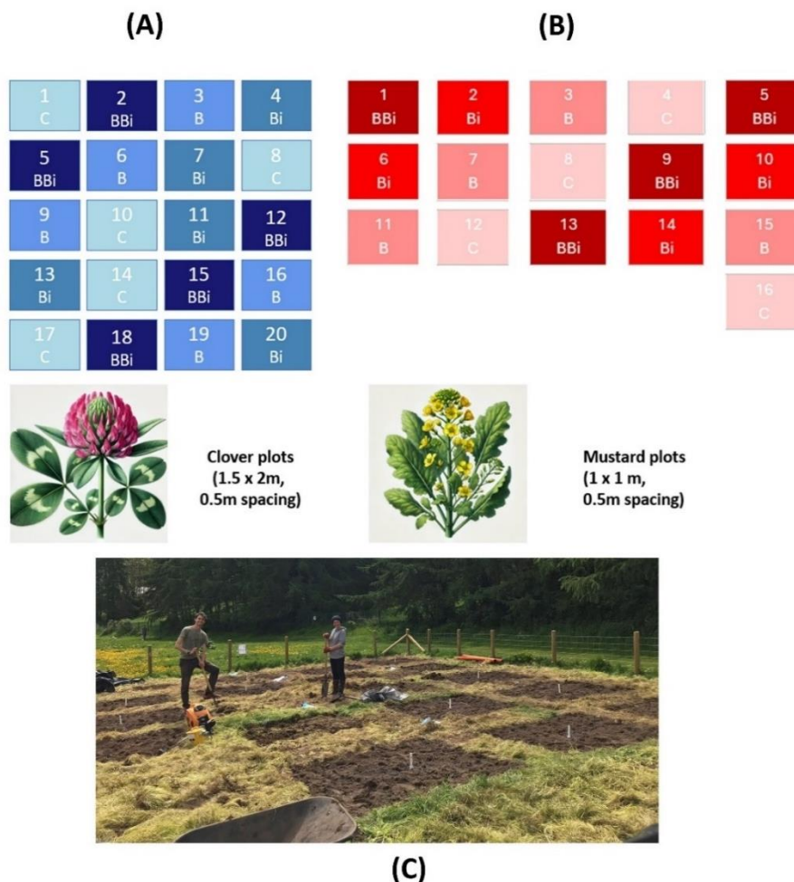
Figure 2: Schematic overview of (A) clover plots and (B) mustard plots with treatments, plot numbers, plot sizes and spacing between plots. (C) Picture of amendment of the clover field plots. The stripped grass plots, yellow mixer to homogenize soils, white TMS TOMST temperature and soil moisture sensors can be identified.
