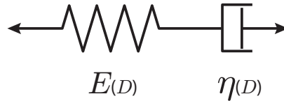
Figure 1. Schematic of the one-dimensional Maxwell model for a continuum material with elastic modulus E and viscosity \eta . Both elastic modulus and viscosity depend on the damage level, D .
