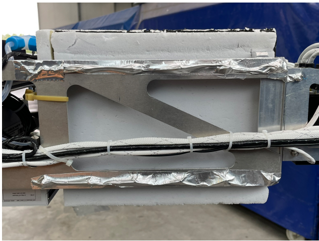
Figure 2. Ozone instrument with insulation as mounted inside the TPC-TOSS in the rear part.
