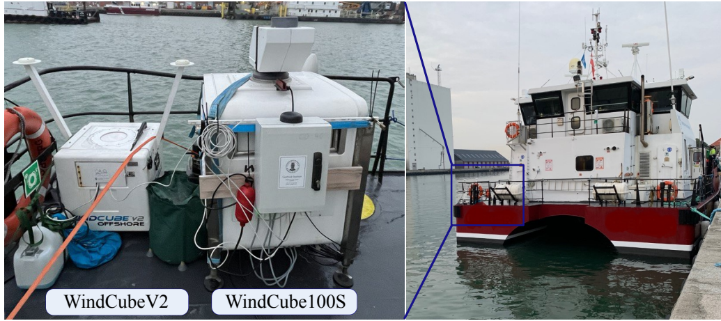
Figure 2. Location of the WindCubeV2 and WindCube100S lidars mounted on the stern of the CTV. Azimuth angles were defined relative to the vessel's heading and corrected using GPS true heading from the IMU.
